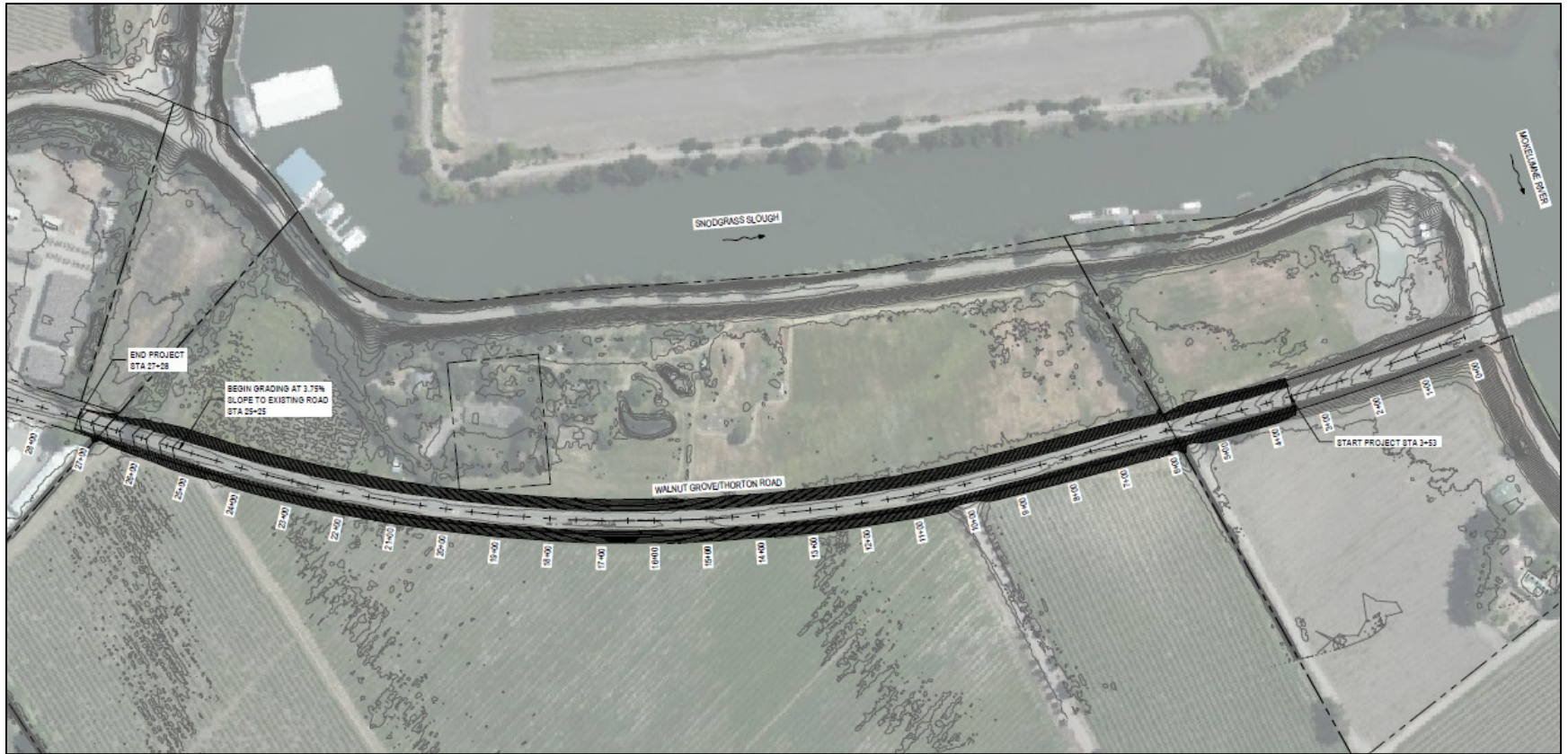
Figure 5-15: Plan View of Proposed Road Widening along Walnut Grove-Thornton Road in RD 563 (Kjeldsen et. al., 2020b)
