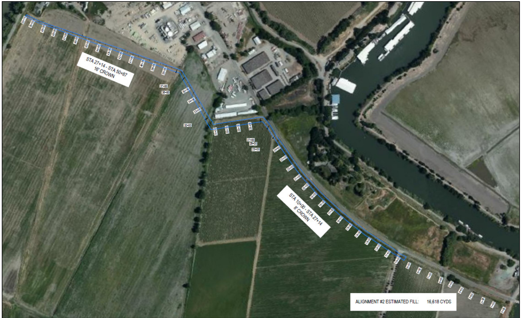
Figure 5-14: Proposed Alignment for the All-Weather Access Road/Flood Fight Berm in RD 563 (Kjeldsen et. al., 2020a)
