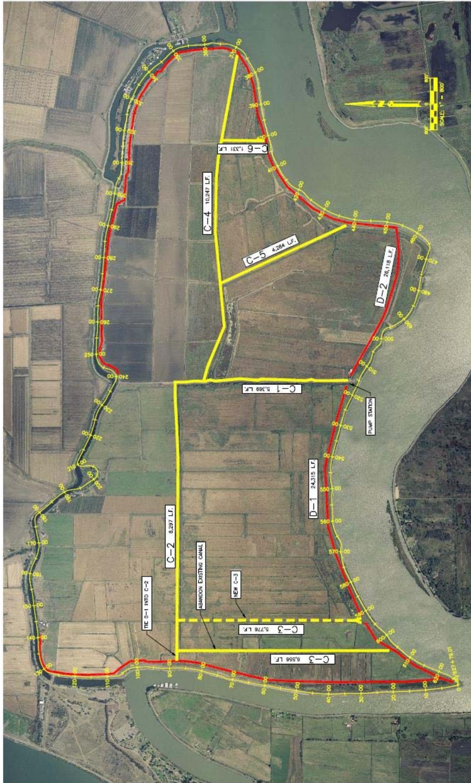
Figure 11-2 RD 1601 Drainage System
