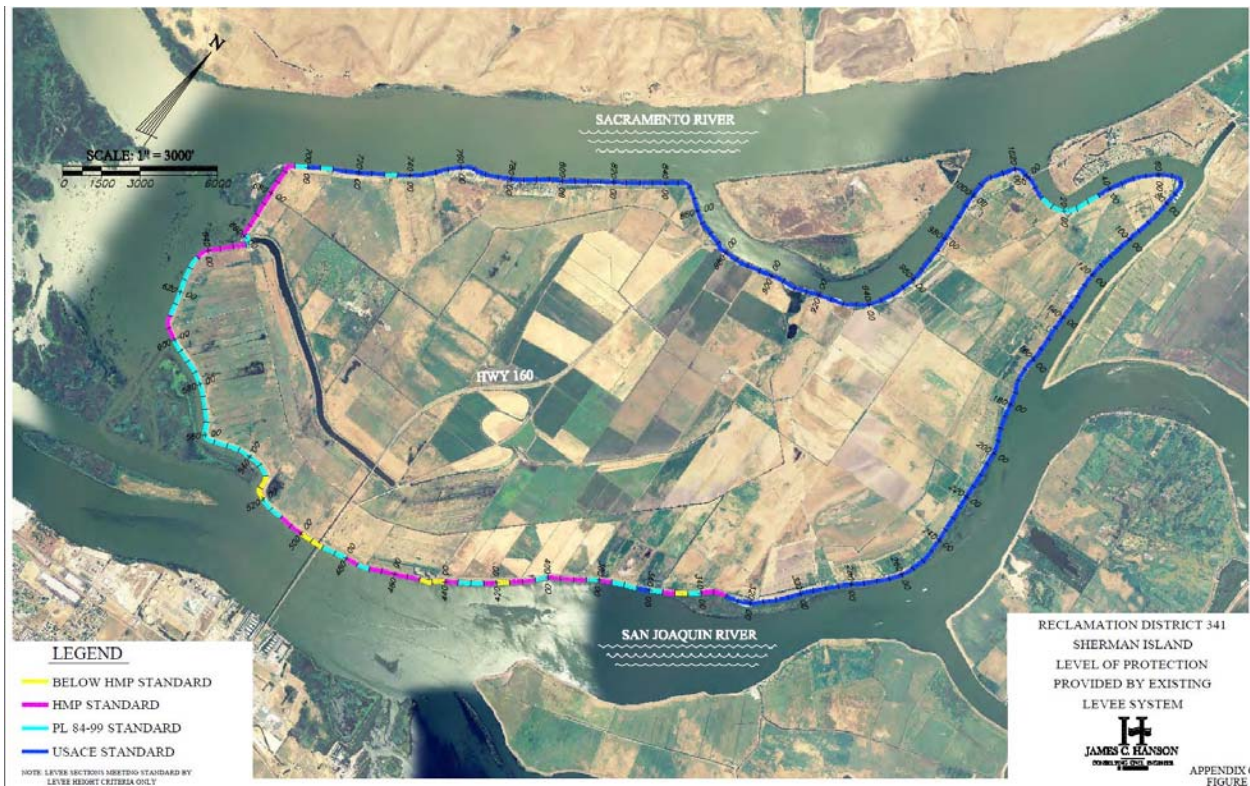
Figure 4-2 Level of Levee Flood Protection in Reclamation District 341
