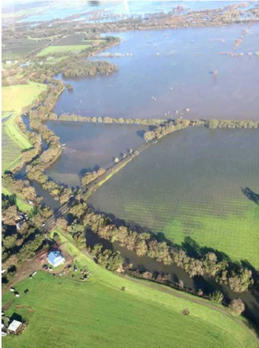
Figure R-18 New Hope Levee Break
