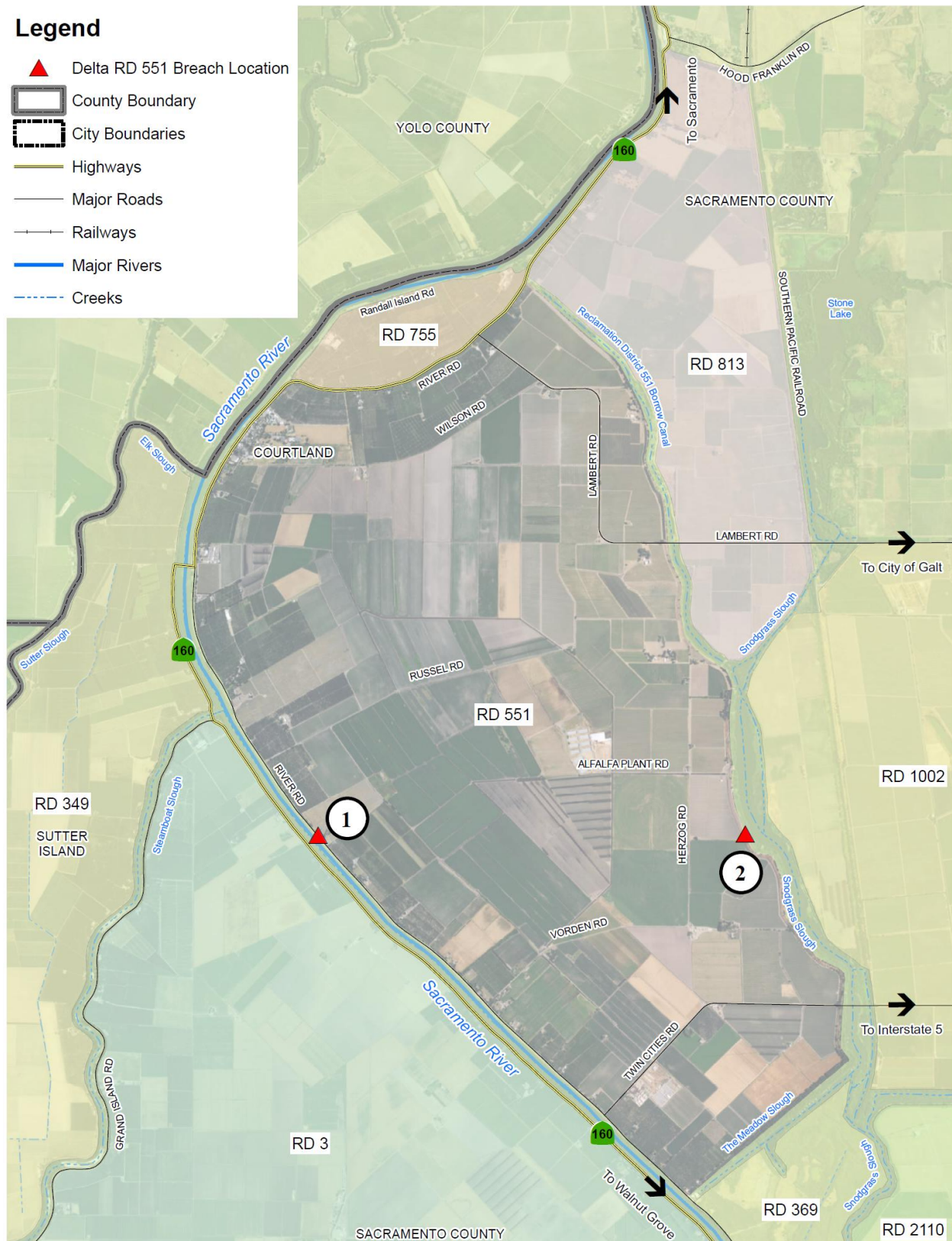
Figure 7-4 RD 551 – Potential Levee Breach Location
