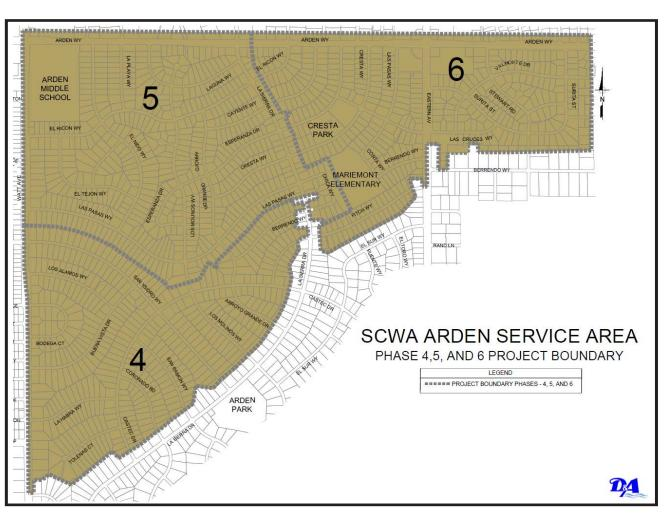
Phase 4, 5 & 6 construction is expected to begin in October 2023. This project will abandon old distribution pipelines located in backyards, install more than 14 miles of new distribution pipelines within street right-of-way, install 1,428 new service lines and meters, install new or replace 145 fire hydrants and 22 backflow preventer assemblies. This Project will provide several critical improvements to the Arden Service Area's distribution system.
