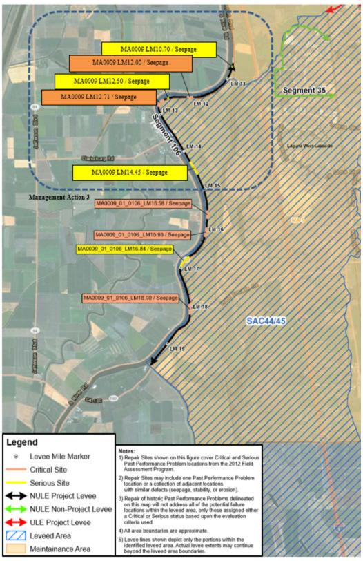
Figure 6-2. Management Action 3 - Repair of DWR FSRP Sites in MA 9 Upstream of Hood Study Area (URS, 2013a), updated in 2020 by Sacramento County
