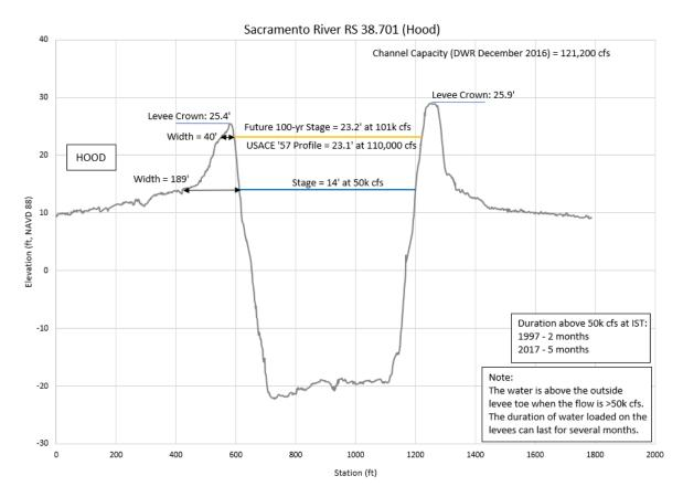
Figure 2-4. Cross Section at Sacramento River Station 38.701 at Hood Viewing Downstream
