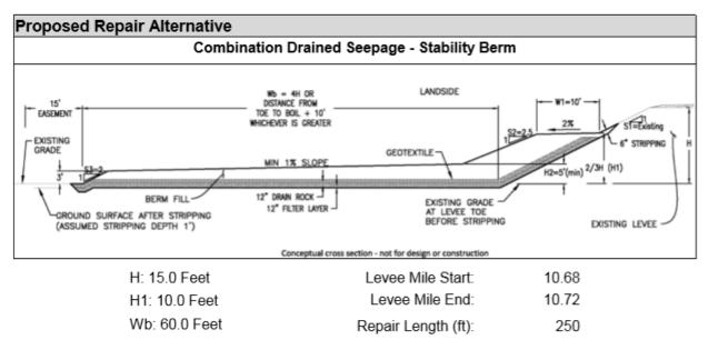
Figure 7-5. Proposed Combination Drained Seepage/Stability Berm Specifications for Repair of Serious Seepage Site Located at LM 10.68 to 10.72 (URS, 2013b).
