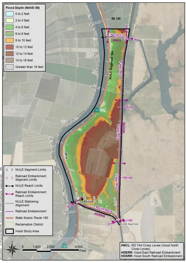
Figure 5-12. Maximum Flood Depths in Hood Study Area Following a Potential Relief Cut of East Railroad Embankment.
