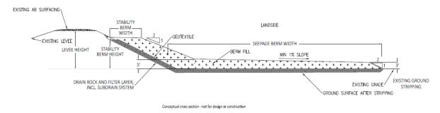
Figure 5-3. Typical Combination Seepage and Stability Berm.
