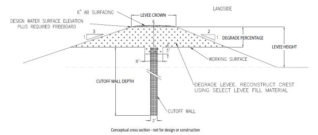
Figure 5-1. Typical Cutoff Wall.
