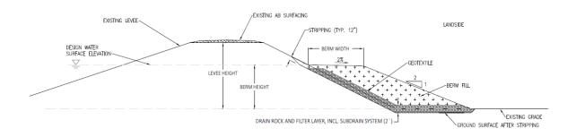
Figure 5-2. Typical Stability Berm.
