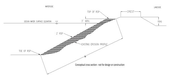
Figure 5-4. Typical RSP Detail to Address Erosion Concerns Within the Study Area
