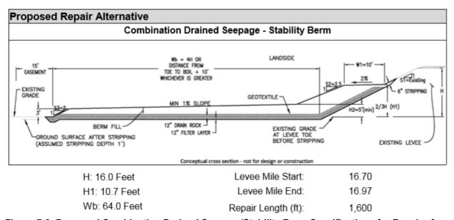
Figure 7-3. Proposed Combination Drained Seepage/Stability Berm Specifications for Repair of Serious Seepage Site Located at LM 16.70 to 16.97 (URS, 2013b).
