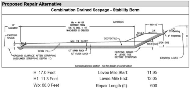
Figure 7-6. Proposed Combination Drained Seepage/Stability Berm Specifications for Repair of Critical Seepage Site Located at LM 11.95 to 12.05 (URS, 2013b).
