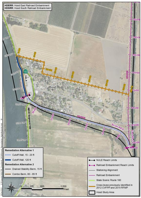
Figure 5-6. Cross Levee North of Hood Paired with; Repair and Strengthen-in-Place MA 9 SPFC Levee Adjacent to Hood; and Repair/ Strengthen Existing Non-SPFC Levee South of Hood (2012 CVFPP and 2014 RFMP Configuration)
