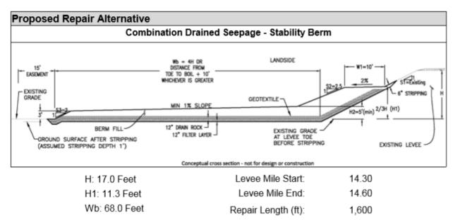
Figure 7-9. Proposed Combination Drained Seepage/Stability Berm Specifications for Repair of Serious Seepage Site Located at LM 14.30 to 14.60 (URS, 2013b).
