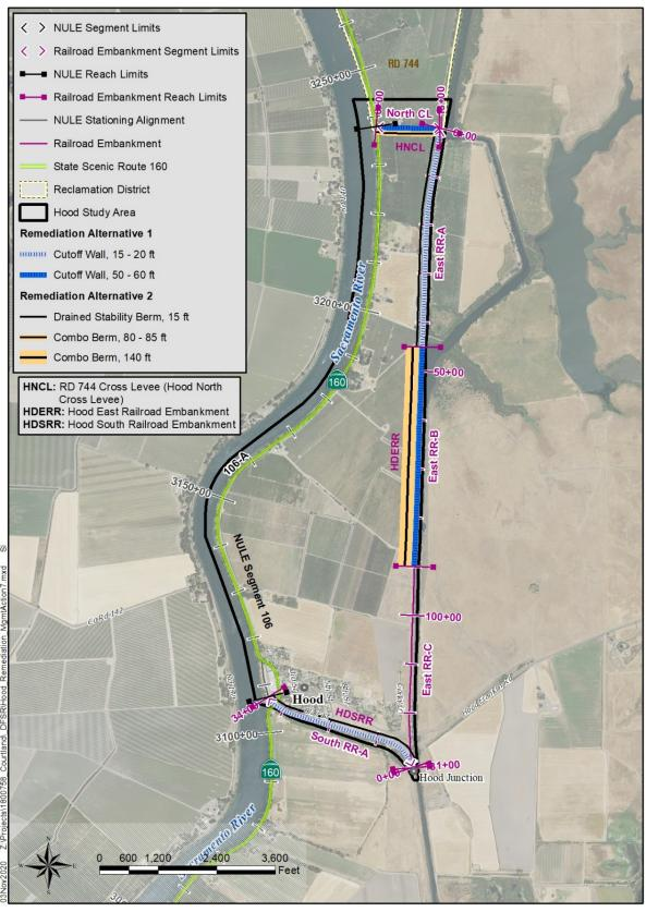
Figure 5-10. Remedial Alternatives to Improve non-SPFC Levee System (former railroad embankments) within the Hood Study Area
