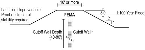
\*seepage cutoff walls are required in most SPFC levees in the North Delta to meet FEMA's current accreditation standards per 44 CFR Section 65.10
